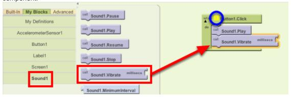
The Sound1.Vibrate block has an open slot, which means you need to plug something into it to specify more about how the behavior should work. Here, we want to specify the length of the vibration. Numbers are calculated in thousandths of a second (milliseconds): to make the phone vibrate for half a second, we need to plug in a value of **500 milliseconds**.
