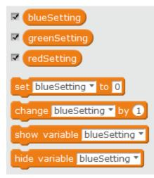
Unless variables are going to be changed early on in a program, it is considered good practice to initialize variables at the start of a program. For my program, I want to start with blue turned on, and green and red turned off. I am going to turn the LEDs on up to a maximum value of 100:
