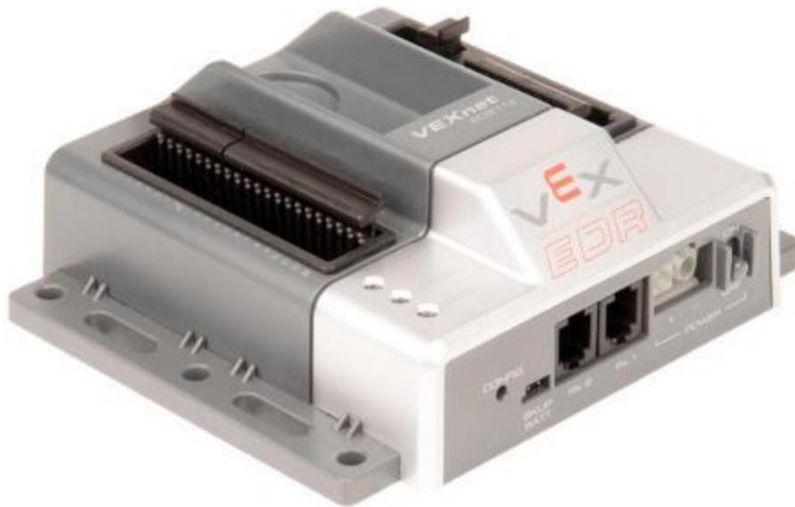
The VEX Cortex Microcontroller comes preprogrammed with a default routine which allows users to get their robots up and running as quickly as possible. With the use of jumper pins, quick adjustments can be made to this default code for greater flexibility. For more advanced programming options, the microcontroller can be fully user programmed using one of the available programming options. More information on these options can be found here: <http://www.vexrobotics.com/products/programming>
