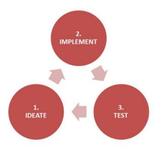
In this simple design loop an idea is generated (1). This idea is <u>implemented</u> (2). After the idea is implemented, the design group would test the product or evaluate the result of the implementation through testing (3). Typically, during this testing and evaluation, additional ideas are generated, and the process starts over again. This cycle and repetition is why it can be said that design is an iterative process.
